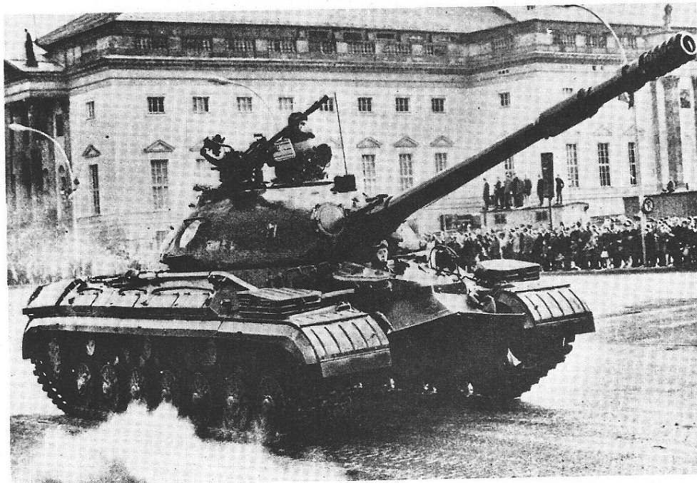
Figure 15-2. T10M tank. (Front view.)
